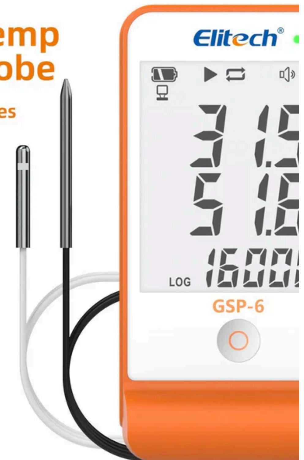
Elitech GSP-6 Temperature and Humidity Data logger conforms to the GSP standard of the new edition. It has one big LCD screen, a button, an External temperature Sensor, and an external humidity sensor. with two modes to save data: Full record stop and cyclic record, the datalogger has the function of over limit sound-light alarm. It can also automatically shorten the record interval in case of over-temperature and humidity limits.
