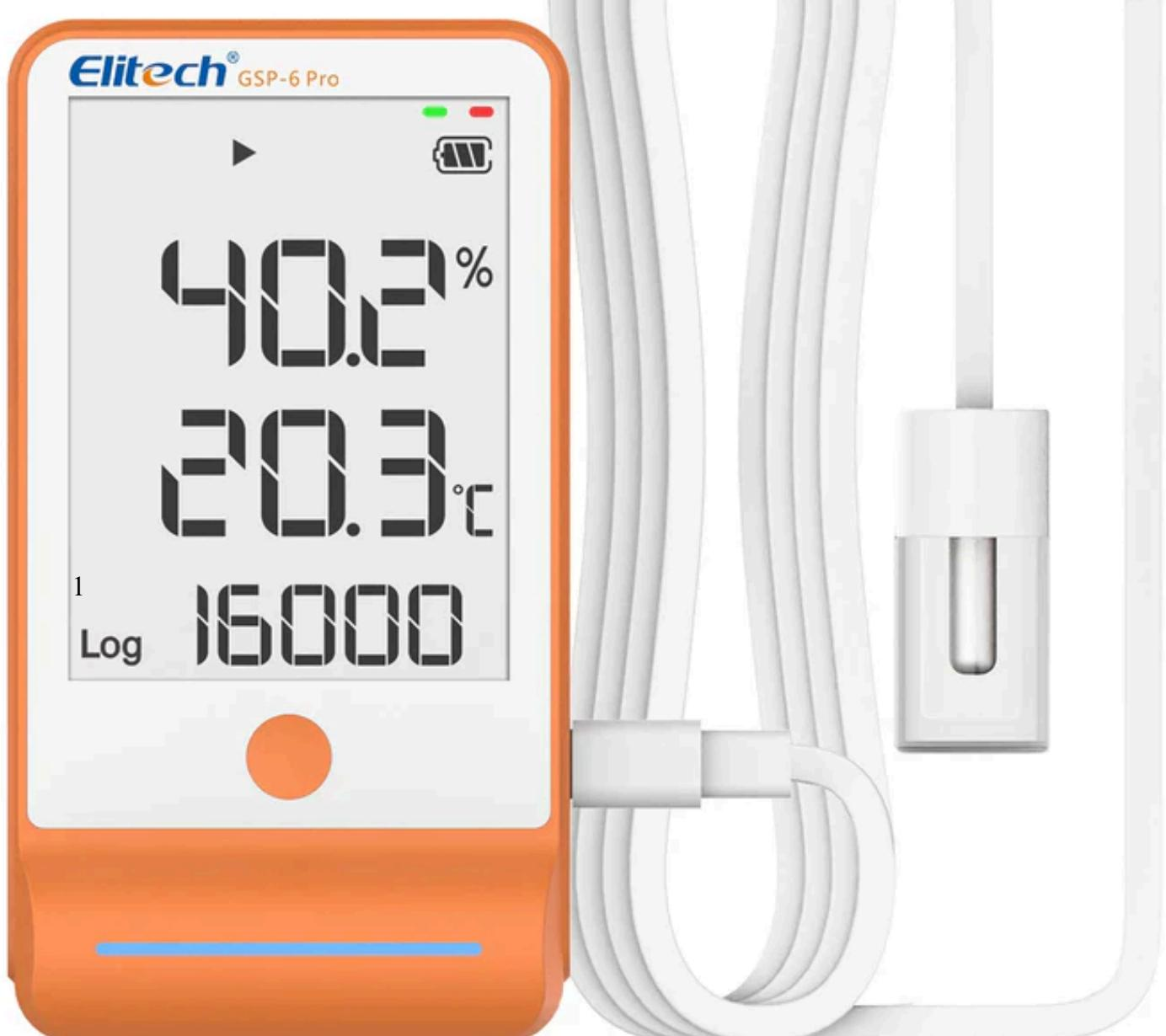
Elitech GSP-6G Temperature and Humidity Data Logger is a multi use data logger designed for reliable temperature monitoring across various applications.
