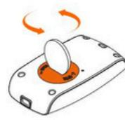
2. Install the battery with "+" side upward and keep it under the metal connector.
